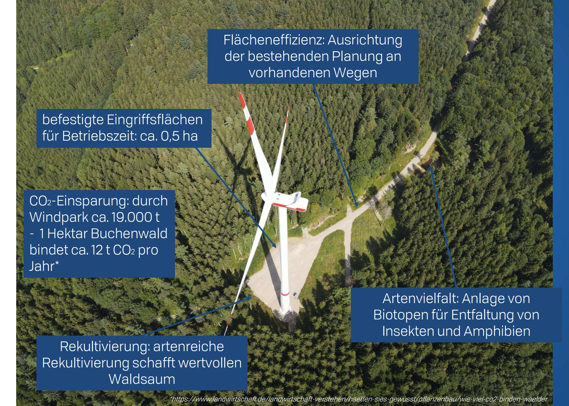
An aerial photograph of a white wind turbine with red-tipped blades, situated in a dense green forest. The turbine is positioned on a cleared area with a dirt path leading to it. Several blue text boxes with white text are overlaid on the image, connected to the scene by blue arrows. The text boxes provide information about the turbine's integration with the forest, its carbon footprint, and the benefits of reforestation.
